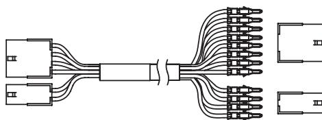
If wood door, order a retrofit cable with the Molex connector on one end, and pins crimped on the other end.
