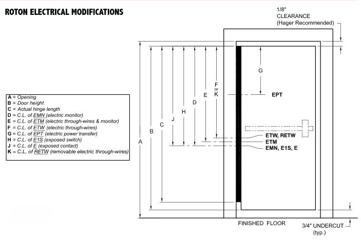
For ease of ordering, Hager Companies has established standard locations for power transfer cutouts. All standard location dimensions are referenced from the top edge of the door to the centerline of the power transfer cutout. Please specify handing.
