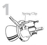
To remove outside knob/lever, remove spring clip with screwdriver (if necessary).
